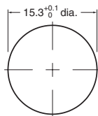
Panel Cutout Dimension Panel thickness = 1 to 4 mm
